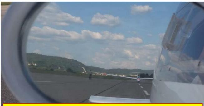
The wing holder must be on the left side of the glider in order to be seen by the tug pilot.
